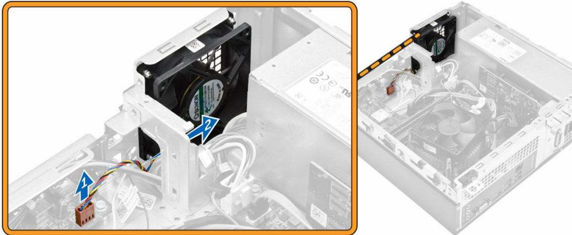
4. Remove the screws that secure the system fan to the computer chassis and remove it from the computer. [1,2]
